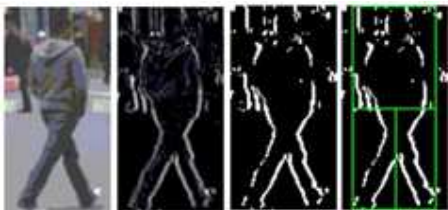
Figure 2. Illustration of the Detection Window Pruning Scheme. The above sequence of figures are sample detection window, magnitude of G_x , edge-linking filtered & thresholded image, three rectangular windows (in green) where number of edge pixels are counted.
